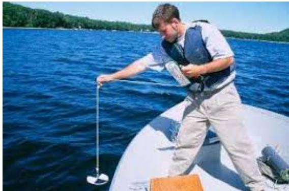
An important indicator of a lake's health is its water clarity. Measuring the clarity is done with a Secchi disk. It is the universal tool used to measure water clarity. The Secchi disk, created in 1865 by Angelo Secchi, is an opaque disc, typically white or black/white used to gage the transparency of water by measuring the depth (Secchi depth) at which the disk ceases to be visible from the surface.
